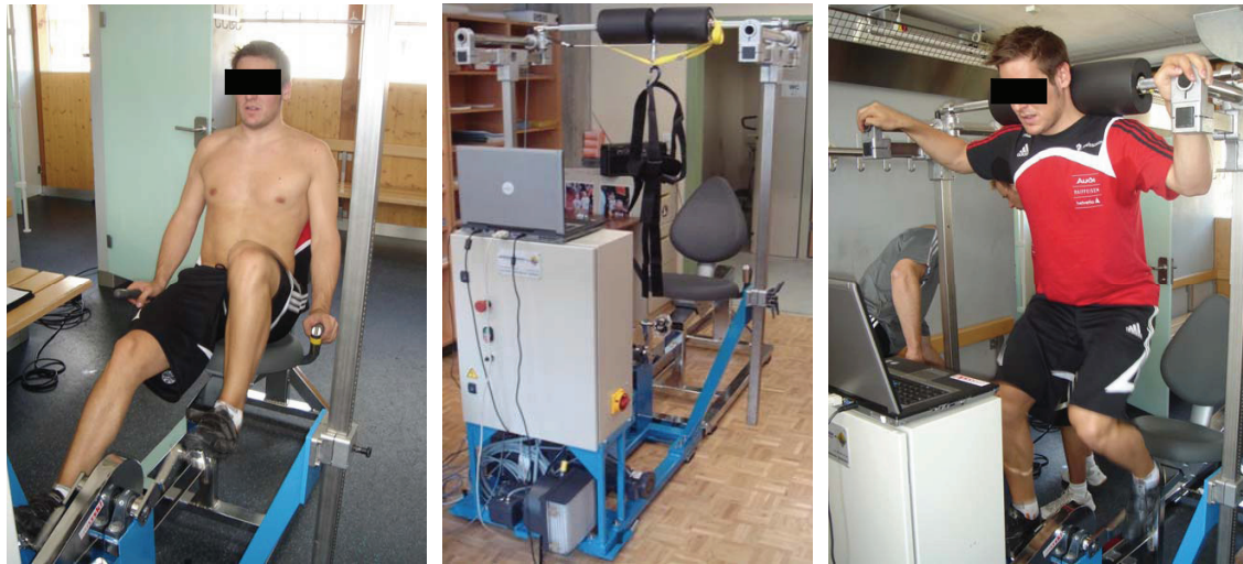
Fig. 3. Eccentric cycle ergometer for training in a sitting position and standing position.
